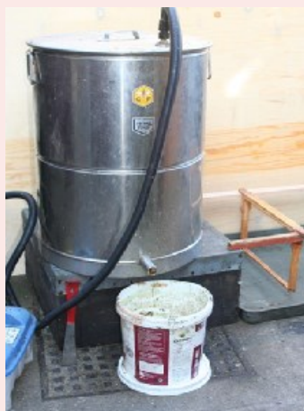
Burco type boiler
